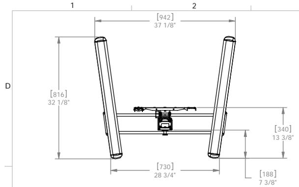
NOTE: CUSTOM INTERAFCE BRACKET NOT SHOWN. THE CUSTOM INTERFACE BRACKET NEEDED FOR YOUR DISPLAY WILL ADD BETWEEN 1/2" AND 2" IN DEPTH AND MAY AFFECT LOCATION OF DISPLAY ON THE MOUNT.
